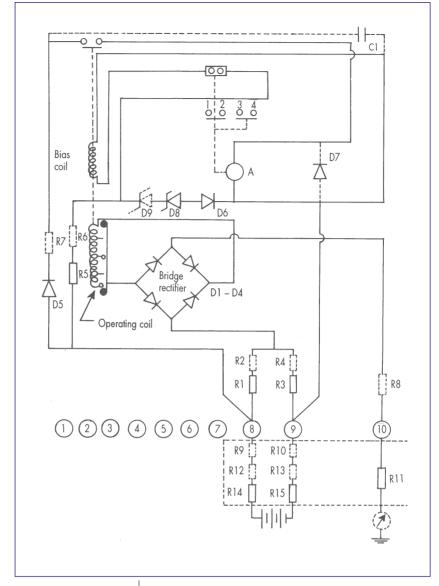
Figure 1: Schematic diagram of external and internal connections for CAEM 21 relay
