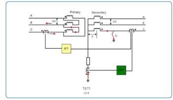
Figure 2: Restricted Earth Fault application
