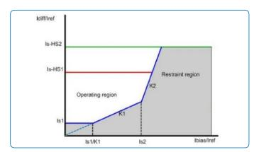
Figure 1: Biased differential protection characteristics
